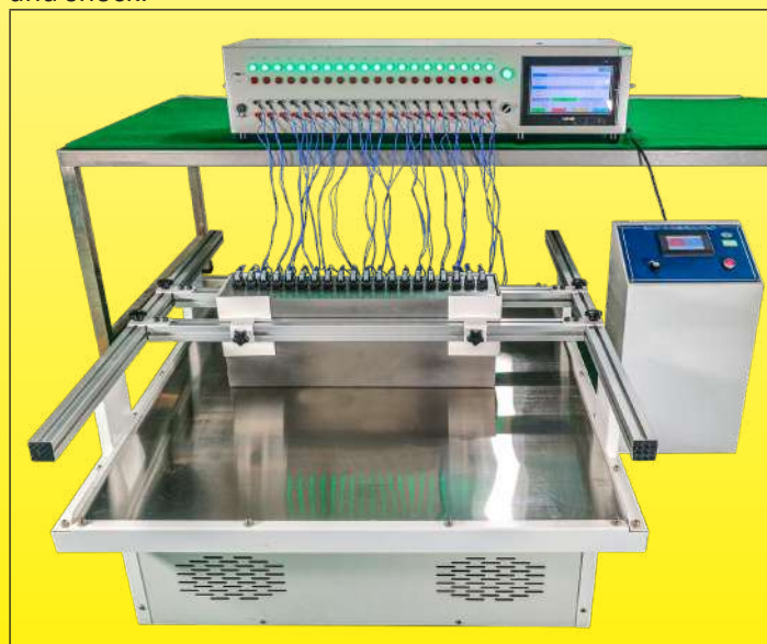
Test equipment to measure the vibration resistance of air switches and slow-action contact of pressure switches by simulation of transport conditions (Ultimheat Laboratory)
