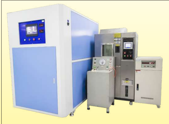
Electrical life test equipment for pressure switches. (Used for verification of compliance with applicable UL and CE standards)
