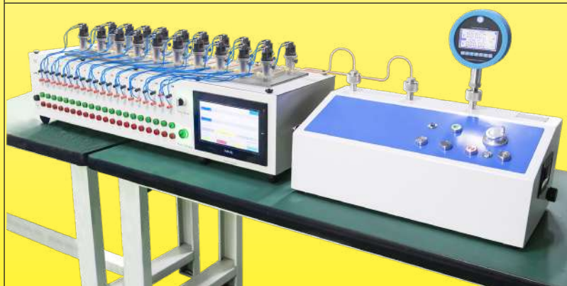
Verification of pressure switch calibration
