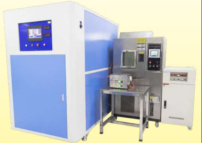
Electrical life test equipment for air switches. (Used for verification of compliance with applicable UL and CE standards)
